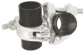
JK-02 SWIVEL COUPLER BRITISH TYPE FOR TUBE OD 48.3mm (EN-74 / BS 1139)
